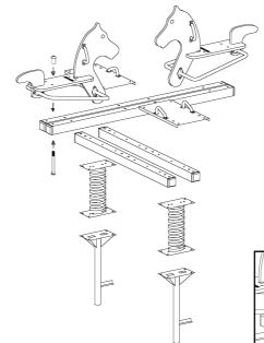
using 130mm cup head bolts and stainless steel cap nuts through the intersecting beams.  $\,$
