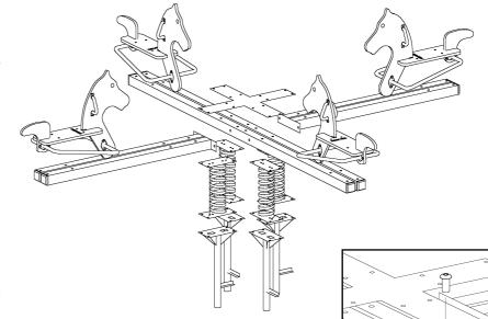
variations. The crossbeams are attached to the main beams using 'tap tight' tri-lobes. The cross plate should be fastened across the top of the beams at the same time the beams are attached to the spring plate using 80mm cup head bolts and stainless steel cap nuts.
