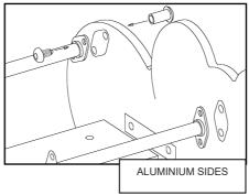
When there are plastic panels use for seat attachment S/S cap nuts with S/S washers  $\frac{1}{2}$ " on panel side and trilobes 10x25 with S/S washers M10 on seat casting side as shown. Use tri-lobes 10x17 and T-nuts for rails as shown
